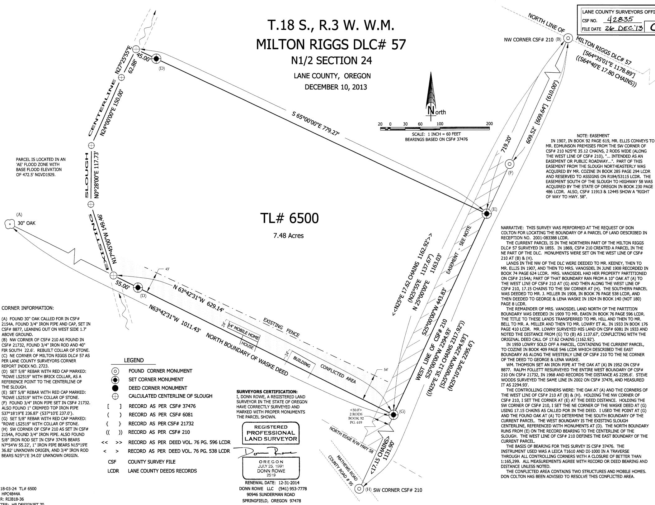
CSF# 210 N25°E 35.12 CHAINS, 2 RODS WIDE (ALONG THE WEST LINE OF CSF# 210), "... INTENDED AS AN EASEMENT OR PUBLIC ROADWAY...". PART OF THIS EASEMENT FROM THE SLOUGH NORTHEASTERLY WAS ACQUIRED BY MR. COZINE IN BOOK 285 PAGE 294 LCDR AND RESERVED TO ASSIGNS ON R184/53115 LCDR. THE EASEMENT SOUTH OF THE SLOUGH TO HIGHWAY 58 WAS ACQUIRED BY THE STATE OF OREGON IN BOOK 230 PAGE 486 LCDR, ALSO, CSF# 11913 & 12445 SHOW A "RIGHT
